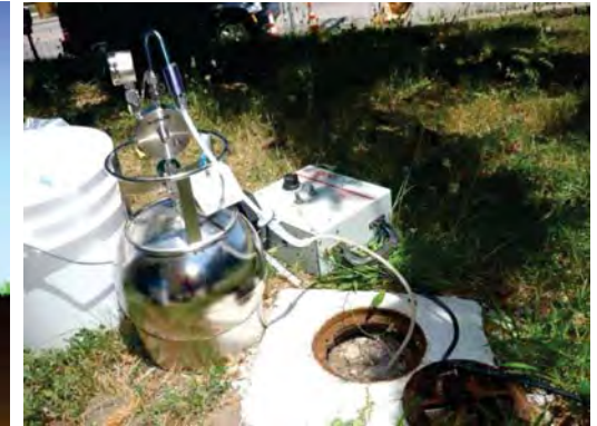
Sampling of a Source Area or Near-Slab Soil Vapor Well
